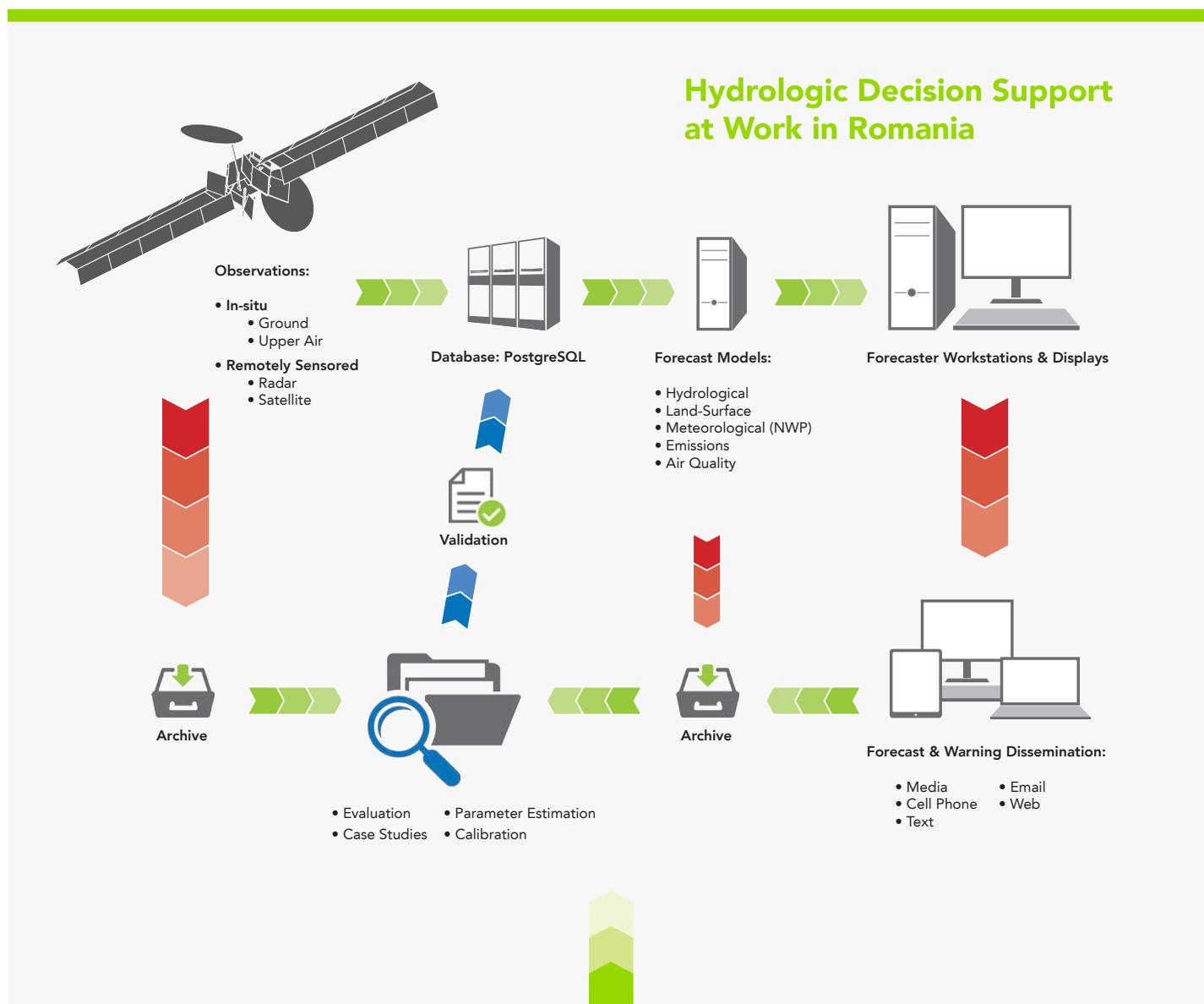
High-level representation of Baron hydrologic monitoring and forecasting solution currently deployed in Romania.
